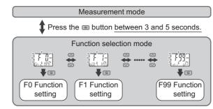
\*: Some products do not have all the functions. If no function is available or selected due to configuration of other functions, [- - -] is displayed on the sub display (right).
